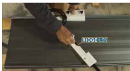
Ridge -LSS. Used for Standing Seam panels to accurately mark angles as needed.
