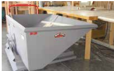
1 yd. "Stretch" Hopper on casters paired with a table saw. Scrap slides directly into the hopper.
