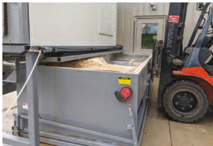
Air powered lid is raised up while hopper is removed to dump
